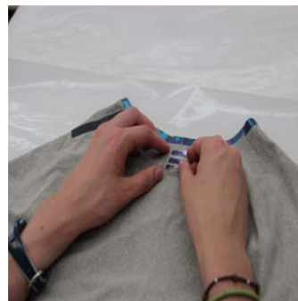
Applying bonded adhesive film
